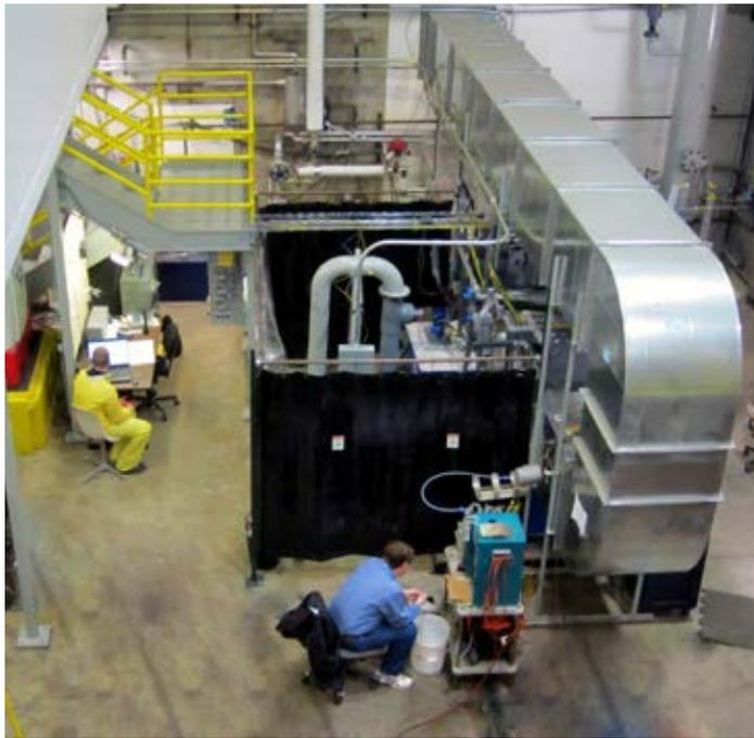
The EERC has designed and built a pilot-scale test facility at its complex in Grand Forks, North Dakota. Procurement and fabrication began in late 2011. After pilot-scale evaluation, future developments will involve long-term testing at a power facility.
